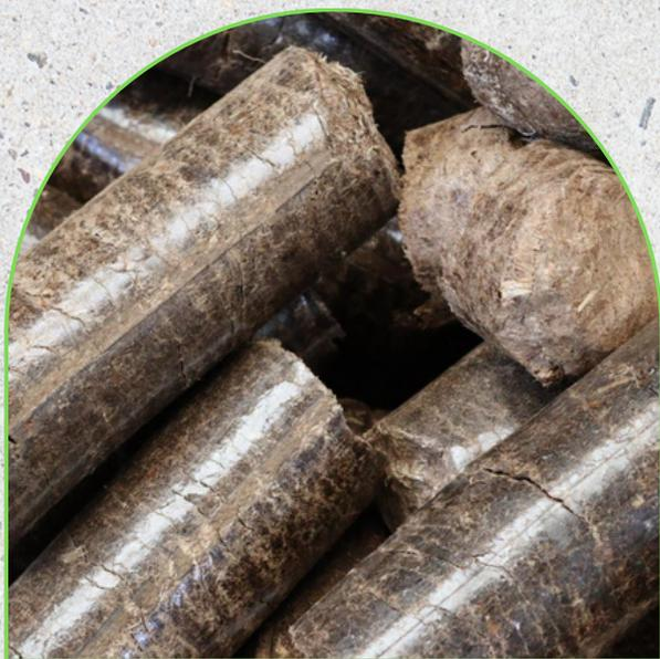
*energy efficient briquettes produced from sugarcane bagasse -
