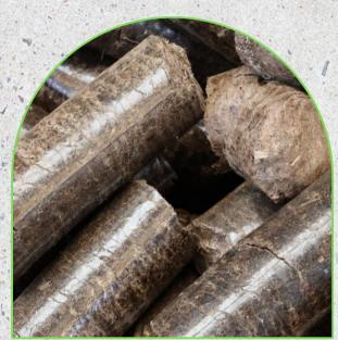
energy efficient briquettes produced from sugarcane bagasse -Acacia Innovations Limited
